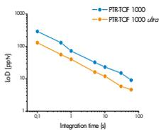
Figure 1: LoDs at m/z 147 for PTR-TOF 1000 and PTR-TOF 1000 ultra for integration times between 0.1 and 60s. LoDs are calculated using the 3σ (standard deviation) method.
