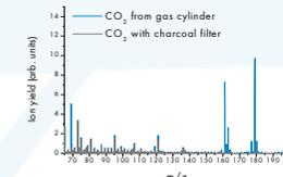
Figure 4: Comparing mass spectra of filtered (=background) and unfiltered CO<sub>2</sub>. Several impurities in food-grade CO<sub>2</sub> are visible.
