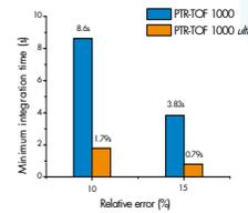
Figure 3: Considerably less integration time (s) needed to achieve a relative error of 10% (15%) for PTR-TOF 1000 ultra than for PTR-TOF 1000, while analyzing a concentration of 100 pptv.
