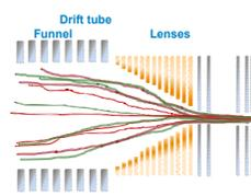
The ion-funnel, consisting of a series of lenses with decreasing apertures and applied RF voltages, focuses the ion trajectories.
