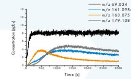
Figure 5: Concentration vs. time. Impurities show different dynamic, which is attributed to their vapor pressure in the cylinder.
