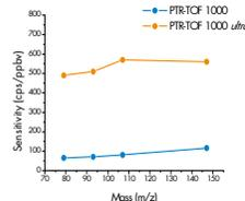
Figure 2: Comparison of the sensitivities for PTR-TOF 1000 and PTR-TOF 1000 ultra. The sensitivities are obtained utilizing compounds from certified gas standards.
