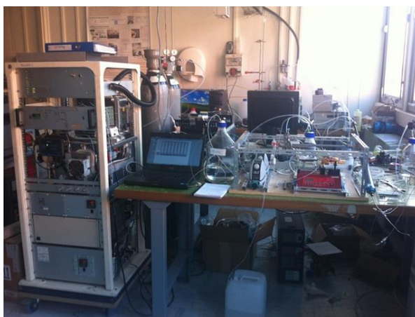
Fig. 1 Ionicon PTRMS coupled to the On Line Water Extraction Device (OLWED) at CEA Saclay, France
